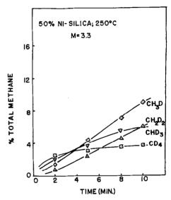
Fig. 2. Methane-deuterium exchange on 50% nickel-Cab-O-Sil, Initial rates shown.
